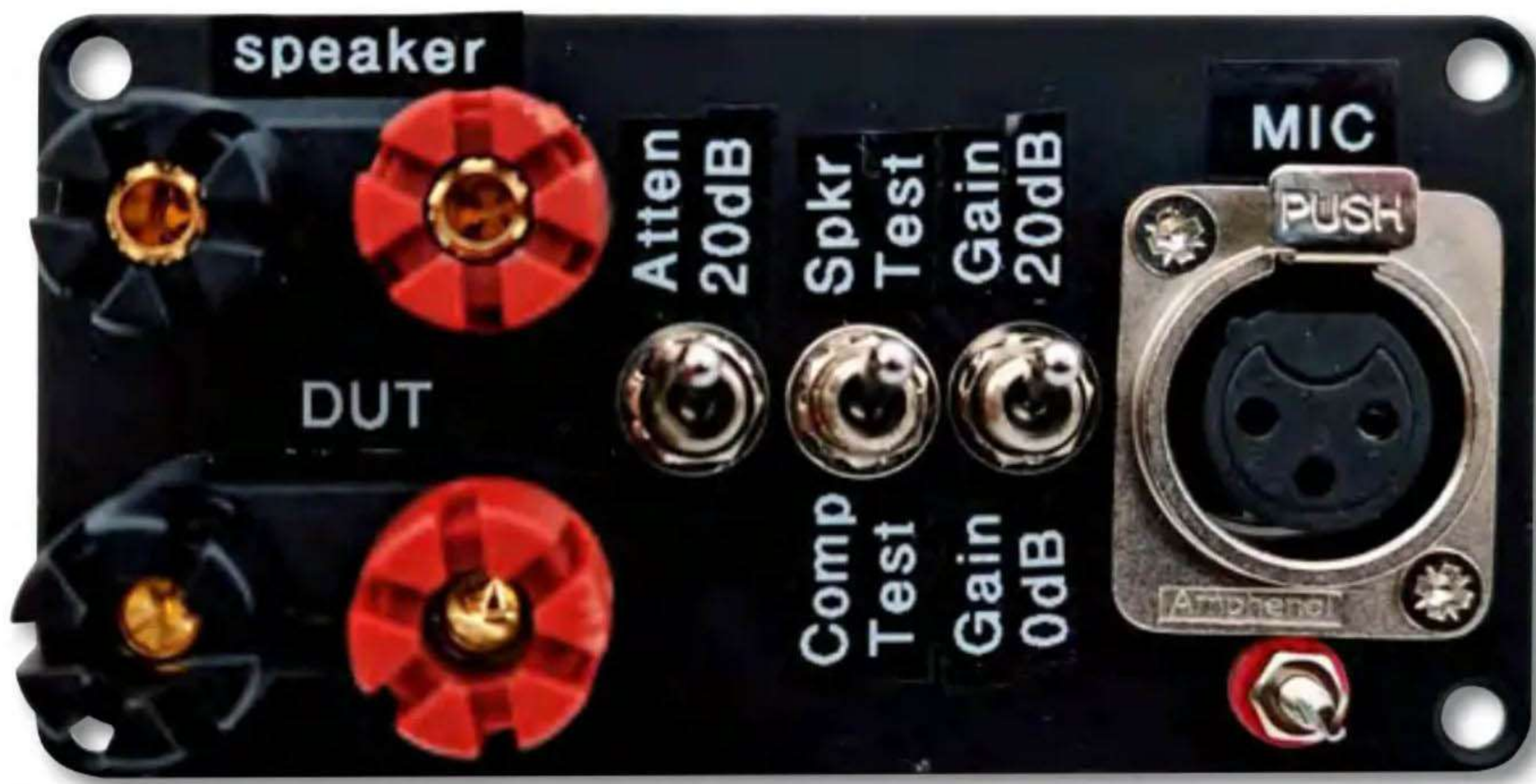
Photo 1: an exterior view of the completed front panel assembly. Dymo labels will help you to remember what each switch and terminal does down the track!
