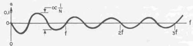
Figure 4. The phase correction portion of the envelope of the spectrum of a tone burst ( N=3 ).
