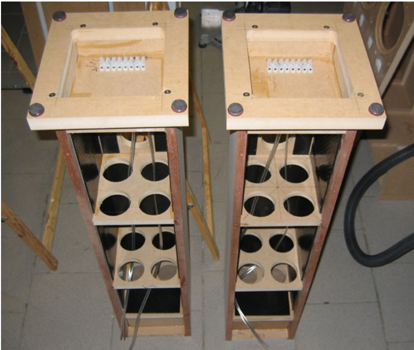
Cabinet bracing and bitumen pads on internal walls. Bottom panel lifted 4 cm allowing crossover to be placed here. Tweeter has it's own chamber.
