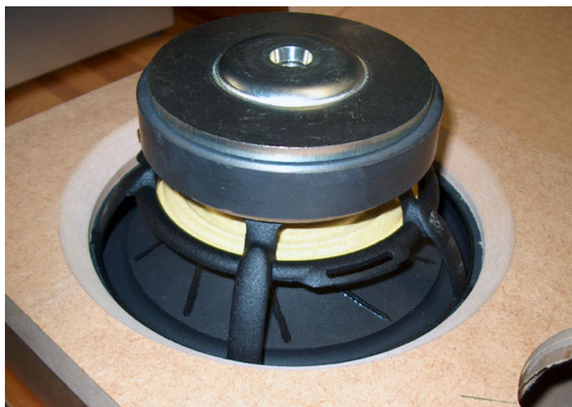
Chamfering of the bass driver hole to provide proper ventilation.
